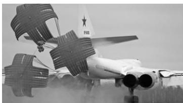
**Fig. 4:** Cross parachutes for deceleration and stabilization
