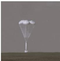
**Fig. 1:** Surface guidance without ribbons parachute
