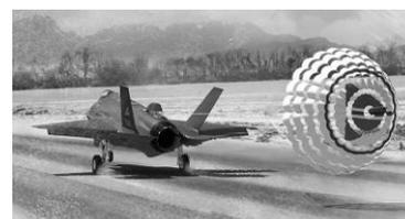
Fig. 7: Annular parachute
