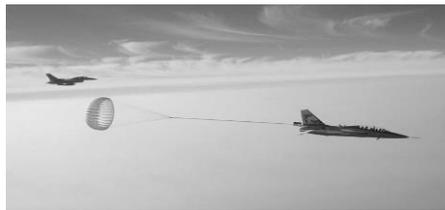
**Fig. 2:** Surface guidance with ribbons parachute
